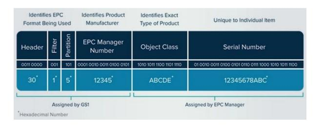
Every RAIN RFID tag includes a unique **160-bit tag identifier (TID)** and *may* include an **electronic product code (EPC)** in its memory banks.
